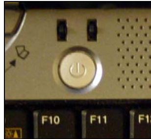
Figure 3.6 On/Off control with bounce back – is it on or off now?
